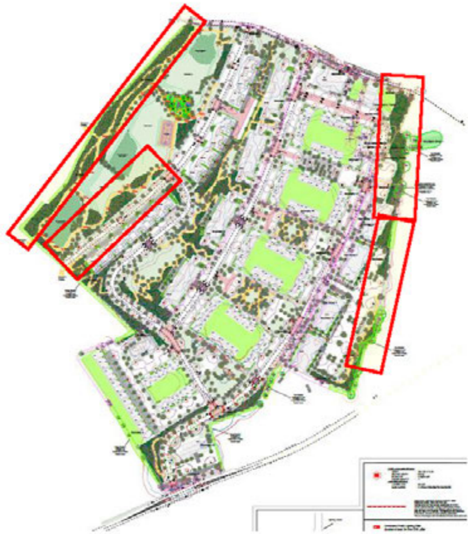
Proposed development layout Areas indicated red boxes must be managed for control of lighting to provide darker areas for bats
